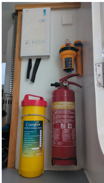
Fire blanket, EPRIB Flares, Extinguisher
