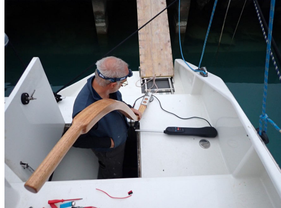
A removable tiller pilot installed on one of Faidapiu's tillers as backup.
